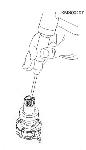
DISASSEMBLING STARTER Disassembling overrunning clutch Slip disassembly sleeve (1) over output shaft and position on stop ring. Knock back stop ring by tapping firmly (plastic-headed hammer) on disassembly sleeve. The following disassembly sleeve is required depending on starter version: - Starter versions with bushing (pinion ID 13.5 mm): 0 986 619 416 - Starter versions with needle bearing (pinion ID 14.7 mm): 0 986 619 407
